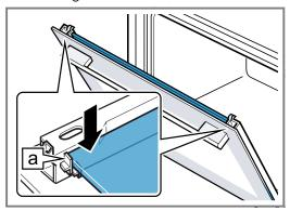
5. Note: When sliding the pane in, ensure that the glossy side of the pane is on the outside and the cut-outs on the left and right are at the top. Slide the inner pane into the left- and right-hand retainers a.
