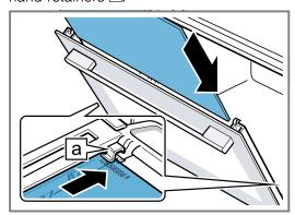
Push the intermediate pane upwards until it is in the left- and right-hand retainers a.
