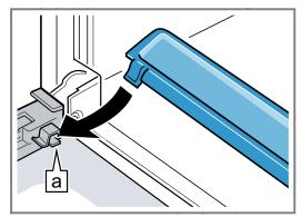
Slide the intermediate pane into the left- and righthand retainers a.
